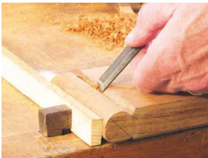
▲ Pic.6 Cleaning up the shoulder with a standard chisel
